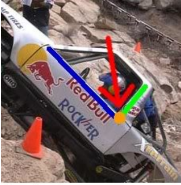
Blue=Doorbar Green=B-pillar Orange=Doorbar Junction to the B-pillar Red=Arrow pointing to the topic of Interest.
